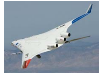
The X-48B Blended Wing Body research aircraft banks smartly during its Block 2 flight phase. (NASA Photo / Carla Thomas)
