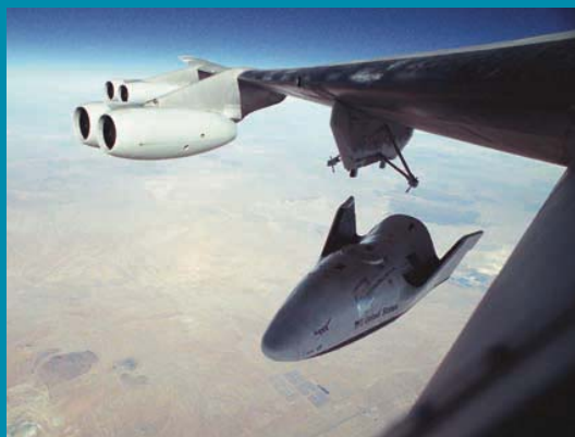
The X-38 vehicle 131R drops away from its launch pylon on the wing of NASA's NB-52B mothership as the X-38 begins its eighth free flight on Dec. 13, 2001.
