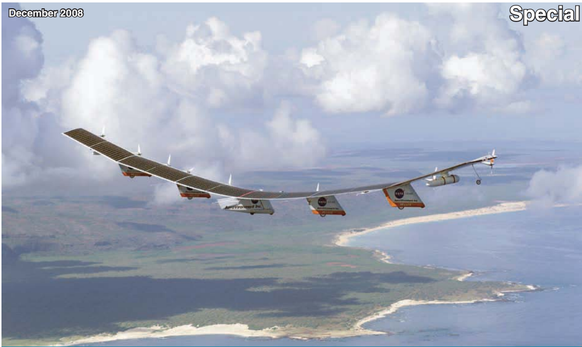
EC03 0152-466 NASA Photo by Carla Thomas NASA's Helios Prototype electrically powered flying wing began a checkout flight June 7, 2003, from the Navy's Pacific Missile Range Facility on the Hawaiian island of Kauai.
