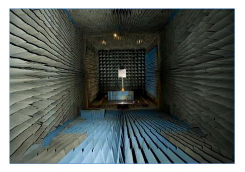
**Above:** The electromagnetically quiet Anechoic Chamber at the Marshall Space Flight Center in Huntsville, Alabama. [larger image]
