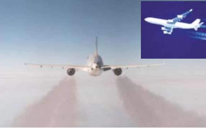
Figure 1. Contrails forming behind the engines of a Lufthansa Airbus A310-330 cruising at an altitude of 35,100 ft (10.7 km) as seen from research aircraft. (Photo: German Aerospace Center (Deutsches Zentrum für Luft- und Raumfahrt (DLR)), Oberpfaffenhofen, Germany.) Inset: Contrails forming behind the engines of a large commercial aircraft. Typically, contrails become visible within roughly a wingspan distance behind the aircraft. (Photo: Masako Imai, Cloud Castle/Photo Sky Japan.)
