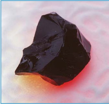
Nicknamed "fast glass," a more efficient formula for vitrifying radioactive waste, was developed by a team of researchers at Pacific Northwest National Laboratory and the Savannah River Technology Center.
