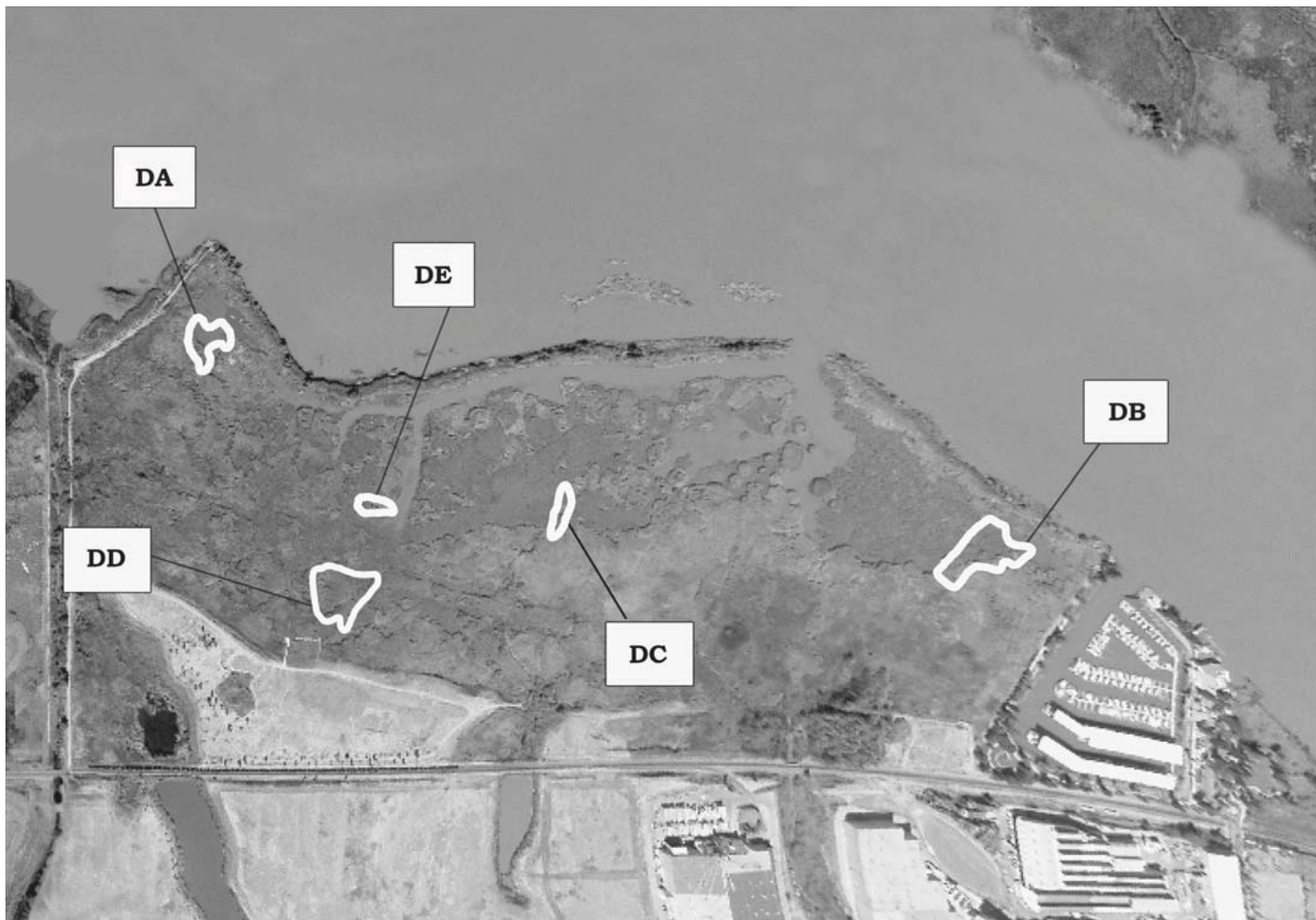
Figure 4. Aerial view of Dow Wetlands, with GIS shape files of the five areas shredded by the Cookie Cutter in 2004 (Table 1).
