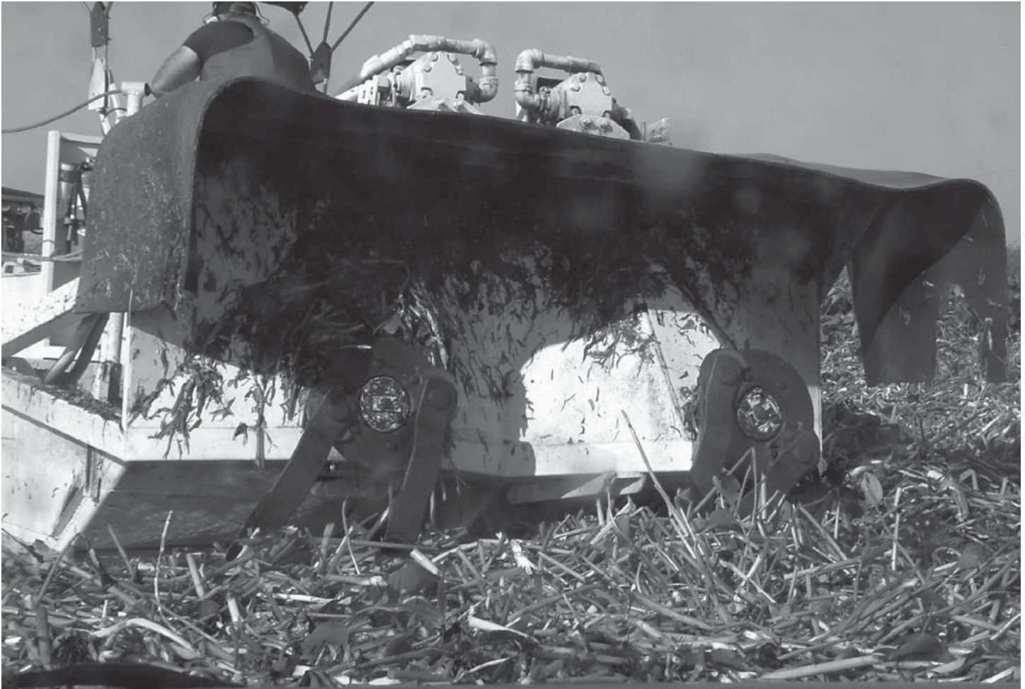
Figure 1. The AquaPlant Terminator, with a view of the rear cutting blades, engine, and cut plant material. Note that there is another set of cutting blades on the front end of the vehicle, which is similar in design to the Cookie Cutter (Figure 3). Photo credit: Bob Case, Contra Costa County Department of Agriculture.
