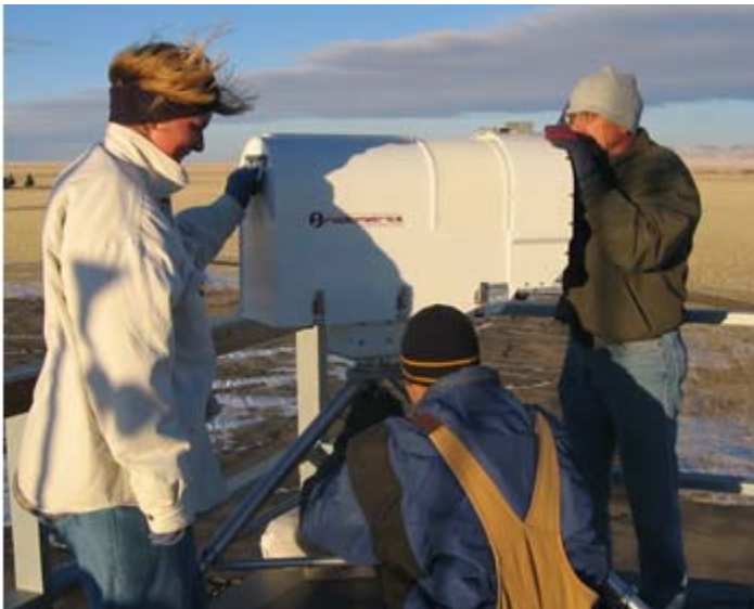
NCAR's Tara Jensen and Dan Breed (standing) align a radiometer with Jason Goehring of Weather Modification, Inc. (Photo by Terry Krauss, WMI.)
