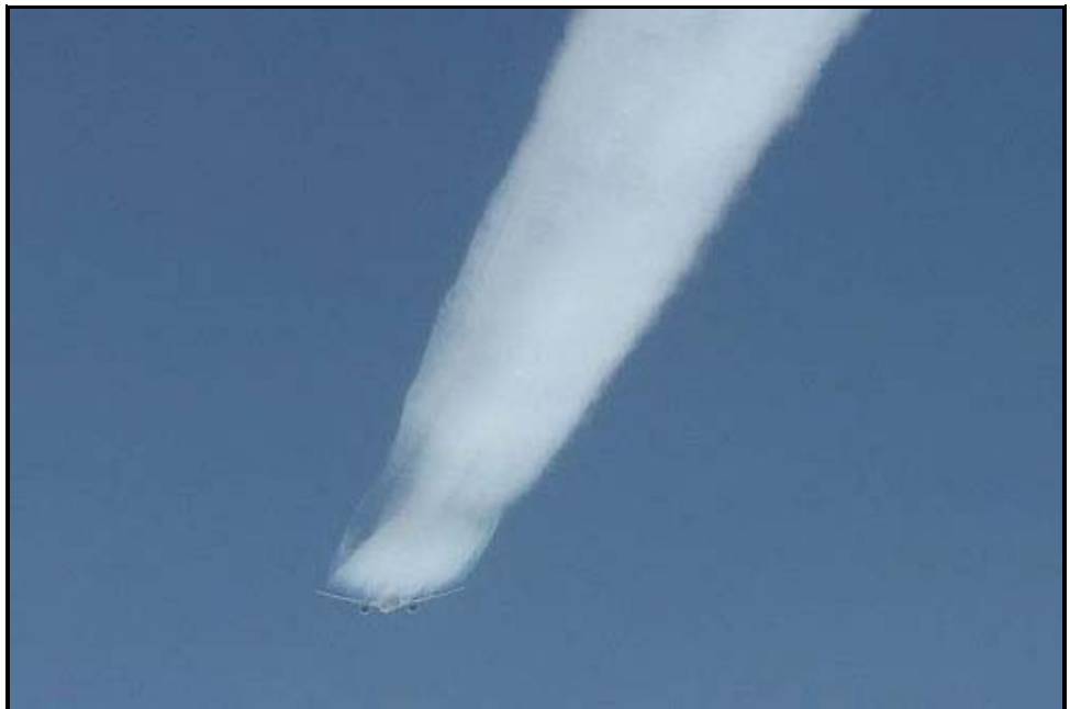
Manifestation of a contrail across the full wingspan of this aircraft.
