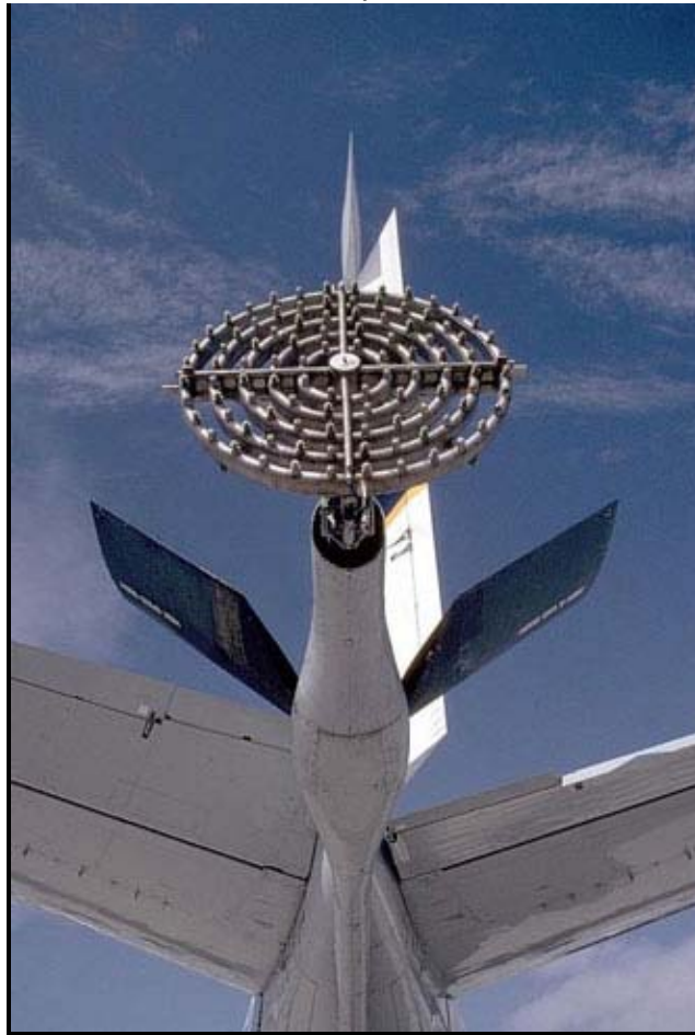
A delivery system of something into the 550 mph airstream... This is an attachment to the refueling boom of a KC-135 or KC-10A tanker. It is also used for inflight de-icing tests.
