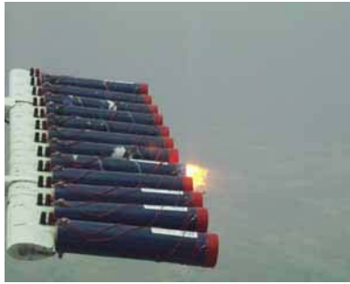
Rack of 12 hygroscopic flares, one recently ignited. Courtesy of National Center for Atmospheric Research/Research Applications Laboratory.
