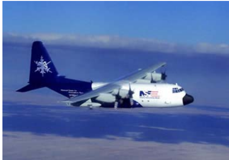
The NSF/NCAR C-130 will fly out of Veracruz, Mexico to intercept Mexico City's pollution plume downwind. A unique array of sensing instruments on board will sample the gases and aerosols in the plume. A four-engine turboprop, the NSF/NCAR C-130 was built for military transport and adapted for research missions in the mid-1990s. (©UCAR, photo by Carlye Calvin)
