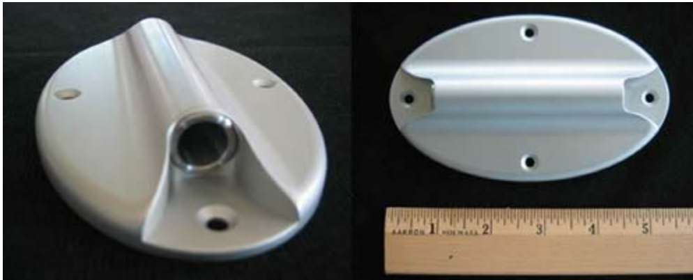
The aerodynamic design of the air sampler removes most ice crystals, particles, rain, and other distractions to improve the sensitivity of the measurement. (Photo courtesy Rex J. Fleming.)
