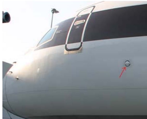
Mounted flush on the side of 25 UPS (B-757) aircraft, the air sampler produces little in-flight drag. (Photo courtesy UPS.)
