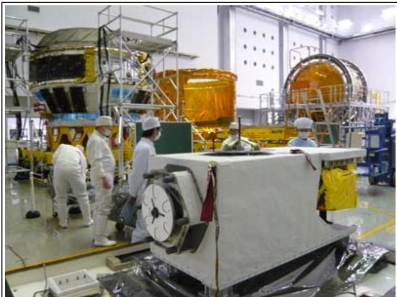
The HICO-RAIDS Experiment Payload (foreground) being prepared for installation aboard the JAXA H-II Transport Vehicle module (background). Source: JAXA
