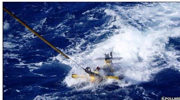
The SeaSoar was used to measure ocean properties down to 300m
