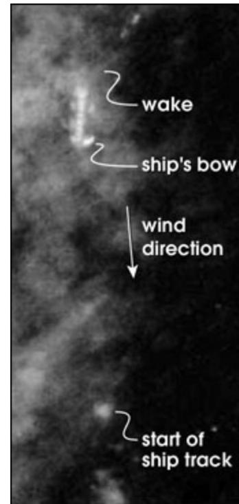
This photograph from a NASA high-altitude research plane shows a ship sailing towards the bottom of the photograph with a ship track blown out ahead of it. The ship track begins about 1,400 m downwind of the ship. (Photograph courtesy Dr. Michael King, NASA GSFC)
