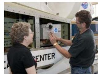
NOAA's Laurel Watts and NASA Dryden's Dennis Pitts install NOAA's Ozone instrument on NASA's Global Hawk. (NASA Photo / Tom Tschida)
