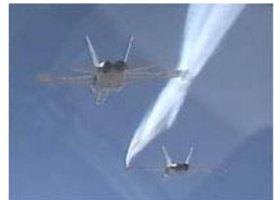
This 32 second video clip shows two F-18s in NASA's Autonomous Formation Flight (AFF) program. The aircraft use smoke contrails to gather data on wingtip vortices. Flight research attempts to utilize the energy in the vortices for more efficient flight. [320x240 QuickTime](#)
