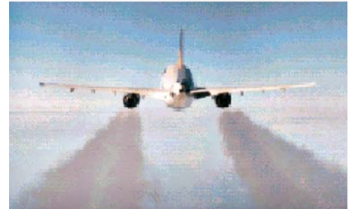
Research aircraft captures this picture of contrails forming behind a commercial jet at 35,000 feet.
