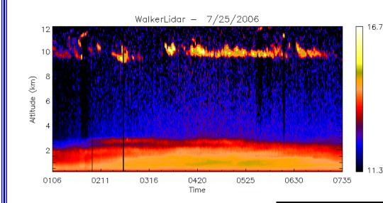
532 nm lidar operated nearly continuously during WAVES
