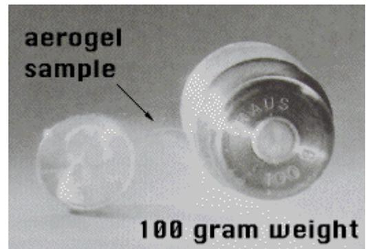
Aerogel is the lightest solid material known - only three times the density of air - and has tremendous insulating capability. However, when made on the ground, it has a hazy or smoky appearance. NASA scientists are experimenting with Aerogel in space and believe that they may be able to learn how to make the foam-like material transparent. A host of new products may result for insulating windows that conserve energy and save money, by lowering heating and cooling costs.
