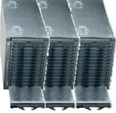
Commercial Blade Processor Example for Pulse compression, Doppler filtering, CFAR detection, tracking, control, etc
