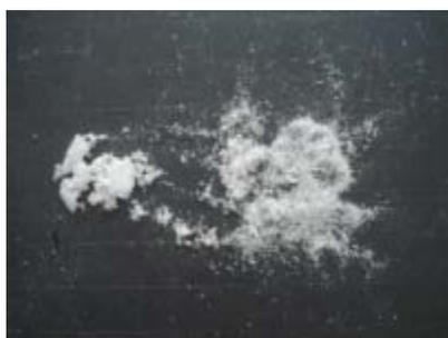
**Polyacrylic acid is added to diapers as a powder (see photo, left) at about 4-5 grams per diaper. It absorbs about 30 times its weight in water, or about 30 mL (1 oz) of water per gram, so a typical diaper can absorb 120-150 mL of water. (See Cool Science for full description on dissecting a diaper.)**
