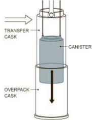
4. A crane lifts the transfer cask directly over the overpack cask. A trap door opens in the bottom of the transfer cask, and the canister inside is lowered into the overpack. A lid is bolted on the overpack which is then hauled outside for storage.
