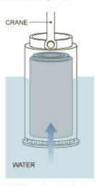
2. When the basket is full, a crane puts a cap on the canister. Then it pulls the transfer cask, with the canister and basket still inside, out of the water and sets it on a stand.
