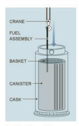
1. After the multipurpose canister has been loaded into a transfer cask and lowered into the water, a crane plucks fuel assemblies from the bottom of the pool and lowers them into the basket.
