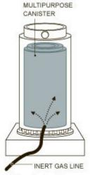
3. A robot welds the top of the multipurpose canister shut. Through a small opening, water is drained out and inert gas is pumped in to prevent corrosion.
