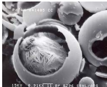
Each microsphere is about 50 microns in diameter, about half the width of a human hair. SRNL originally developed the microspheres as a solid-state storage method for hydrogen as part of the Lab's support of DOE's nuclear defense mission.
