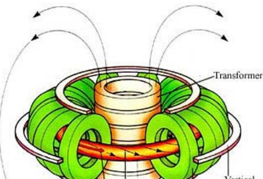
Two magnetic fields combine to produce the **Resultant** magnetic field (labeled left) that spirals helically around the tokamak's torus (orange skinny donut). This Resultant field contains and controls the plasma. The two magnetic fields that combine vectorially to make the Resultant field are: 1) the toroidal field, generated by the green **Toroidal** coils; and 2) the poloidal field generated by the orange **Plasma Current** in the torus. The **Vertical** coils (the large rings around the
