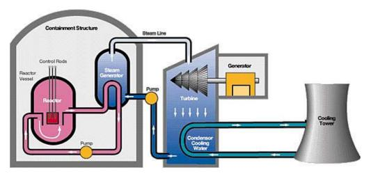
Neutron Fission Power Reactors (NFPRs) are more often called Nuclear Power Reactors, but this commonly accepted terminology is ambiguous because it does not properly distinguish between fusion and fission; and the difference is important. NFPRs (Neutron Fission Power Reactors) get their energy from uranium fission:
