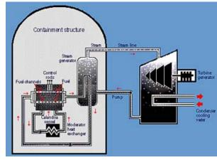
use natural Uranium as a fuel, rather than enriched Uranium. Using heavy water or graphite as a moderator to better optimize the speeds (cross-sections) of the neutrons makes this possible. With only two notable exceptions, most of these reactors have functioned for many years without incident. Nevertheless, many people have serious concerns about them.
