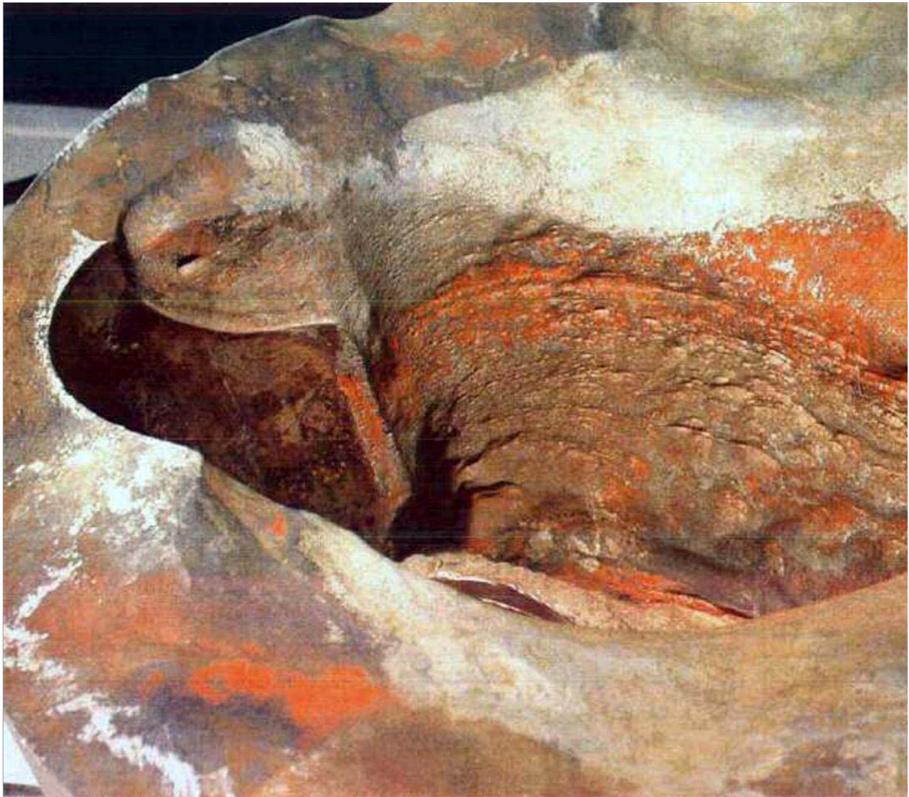
This undated photo made available by the Nuclear Regulatory Commission shows a 5-by-5-inch hole in a section cut from the top of the reactor vessel at the Davis-Besse nuclear plant in C 2002, the hole was eaten by boric acid that spilled from inside the reactor through cracks in the vessel head. Only three-eighths of an inch of steel cladding remained, making a reactor brea months, by the NRC's estimate. (AP Photo/Nuclear Regulatory Commission)
