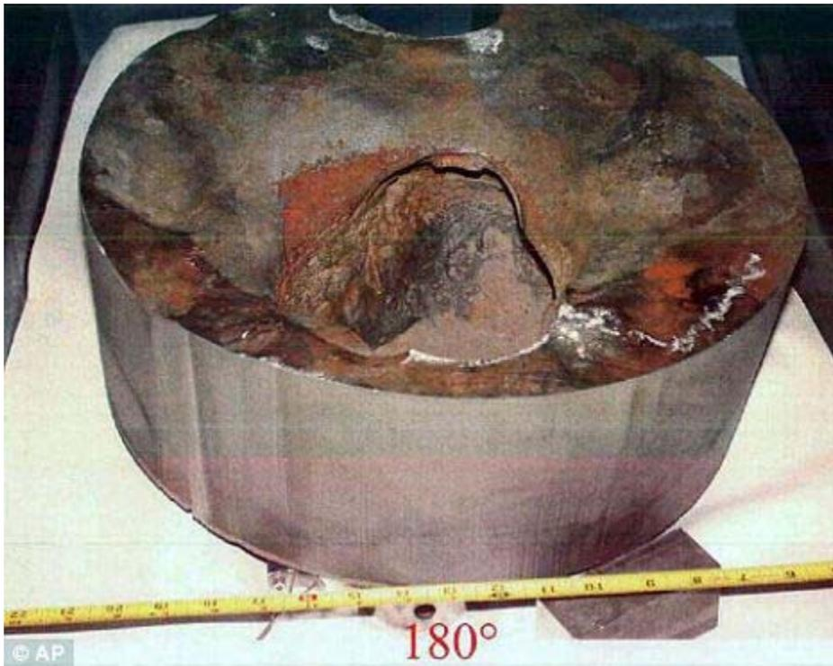
This undated photo made available by the Nuclear Regulatory Commission shows a 5-by-5-inch hole in a section cut from the top of the reactor vessel at the Davis-Besse nuclear plant in Ohio
