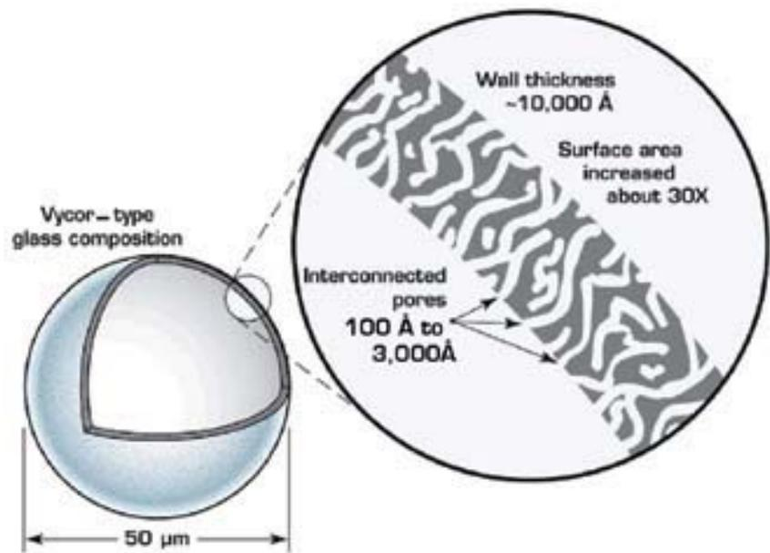
Fig. 2 Schematic representation of SRNL microsphere and wall porosity.
