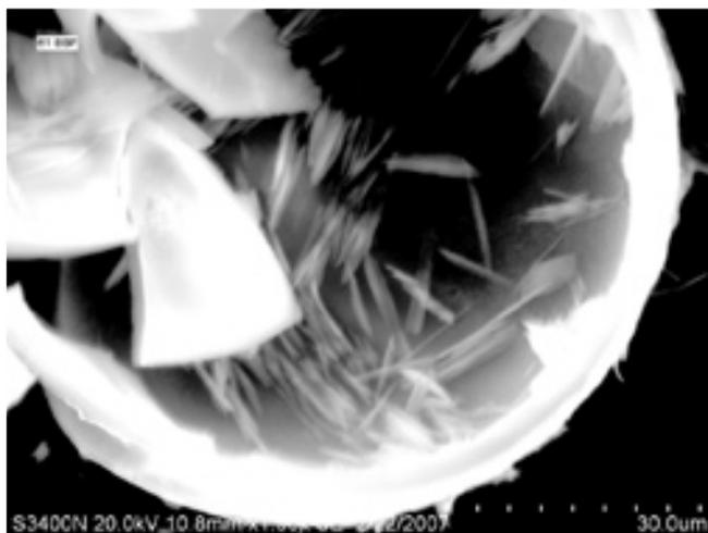
Fig. 6 Nanostructure absorbent grown inside PW-HGMs.
