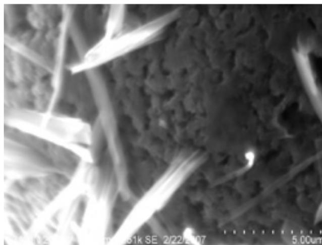
Fig. 7 Nanostructure absorbent grown outside PW-HGMs.
