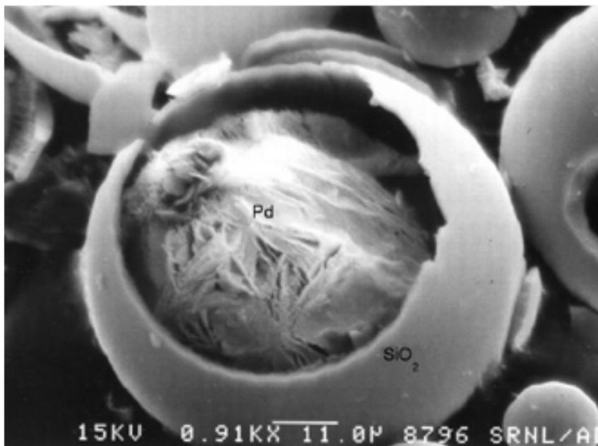
Fig.4 SRNL microsphere filled with palladium where the top of the microballon has been removed to view the inside.
