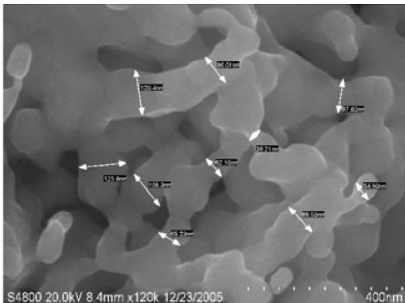
Fig. 5 Unique nanoscale wall porosity through the thin microsphere walls.
