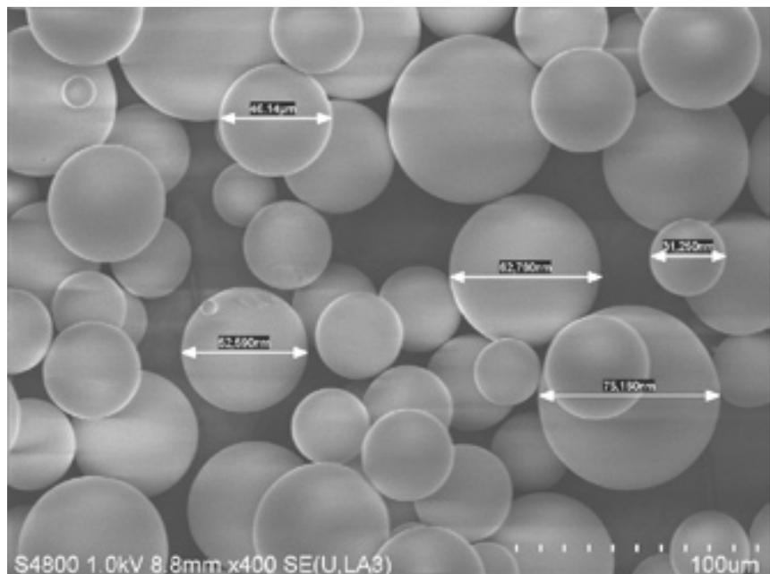
Fig. 3 Typical batch of  $2\ \mu\text{m}$  to  $100\ \mu\text{m}$  with average diameter of  $\sim 50\ \mu\text{m}$  SRNL microspheres.
